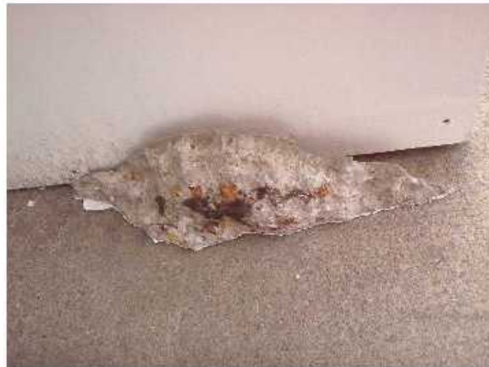
Photo no 5. Close-up of Fascia beam GL 1 F-G concrete spall sample.
