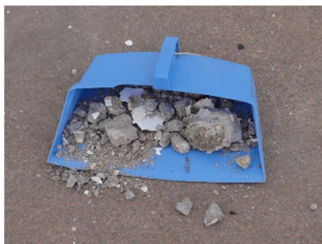
Photo no 8. Close up of spalled concrete from Half-lap joint on fascia beam GL 1, G-H
