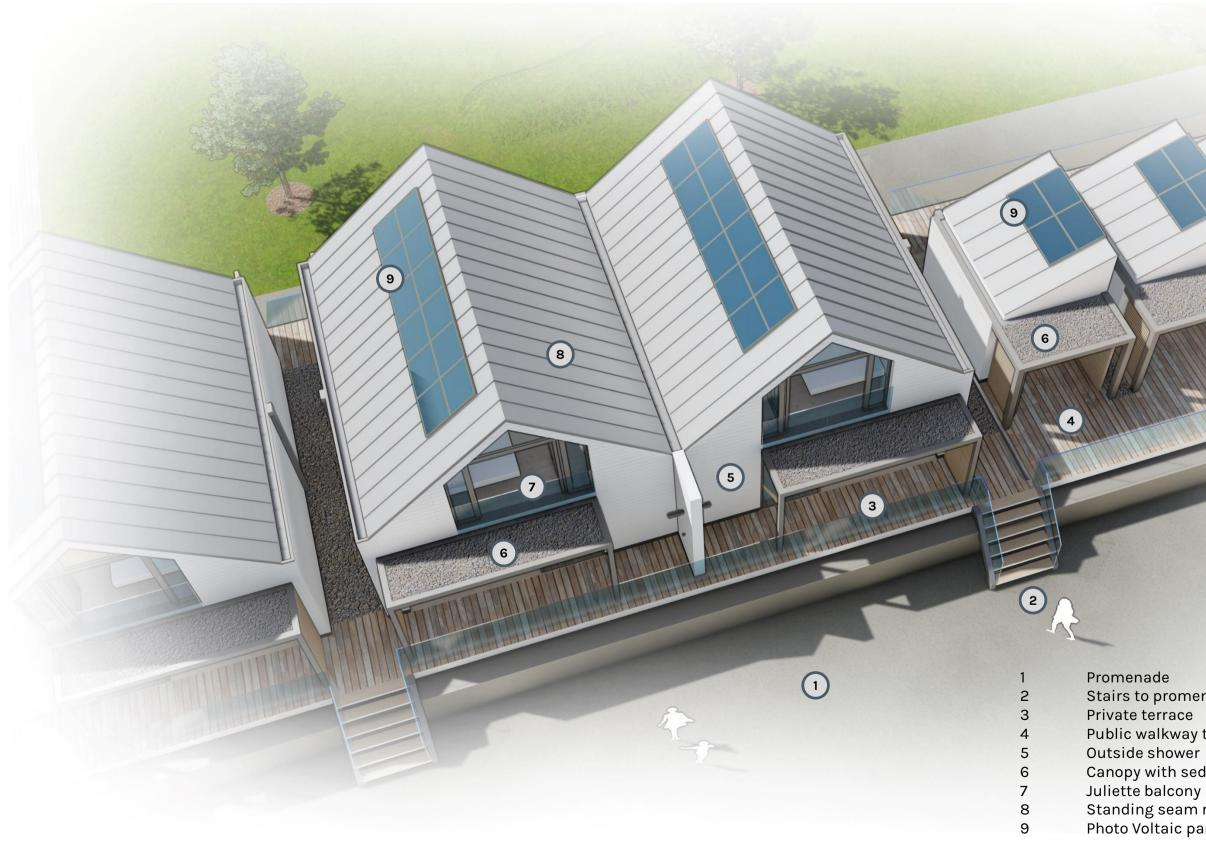
Stairs to promenade level Public walkway to huts Canopy with sedum roof Standing seam roof Photo Voltaic panels
