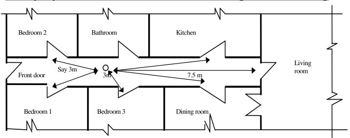
Each alarm should preferably be fixed to the ceiling in a central position and at least 300mm from any wall or light fitting. If the unit is designed to be wall mounted, it should be fixed above the level of the doorway opening in accordance with the manufacturers instructions.
