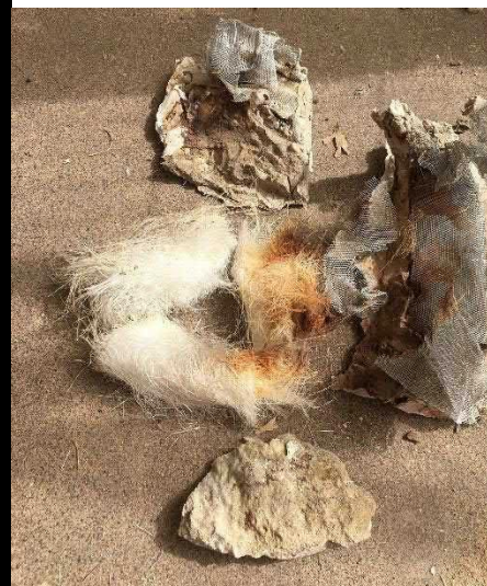
Photo No 06. Debris from previous repair to Half-lap Joint Fascia Beam GL 1, G-H
